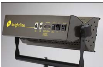
Rear of DMX Fixture (L to R) DMX Thru AC In, Address Selector, On/Off Switch, Power In & Thru
